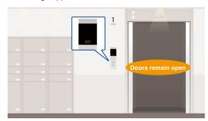
\* The REST indicator remains lit during Fire Emergency Return operation, indicating that the elevator is out of service.
