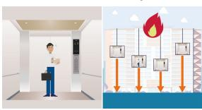
The elevator stops at the evacuation floor, and the passenger evacuates.
