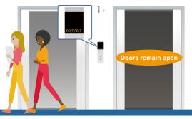
\*The REST indicator remains lit during fire emergency return operation, indicating that the elevator is out of service.
